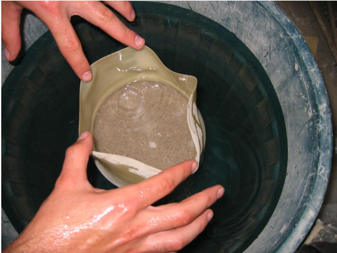
Figure 2 – Soaking sample for saturated undrained RLT test.
